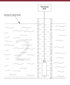
As shown in picture 1, when the sensor is installed in static water such as in poos, water towers, probe is immersed into the bottom and should be as far as possible away from the pump or valves. The terminal box should keep above water surface and prevent water penetrating into cables. Please make sure the airway not be blocked.
